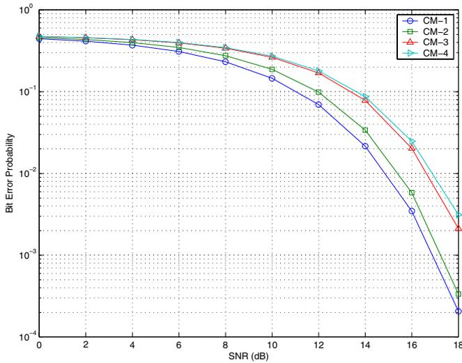
Fig. 3. BEP versus SNR for different IEEE channel models. The parameters are  $N_f = 3$ ,  $N_c = 100$  and  $\Delta = 50$ .  $Q = 10, 20, 50, 50$  for CM-1, CM-2, CM-3 and CM-4, respectively. Average BEPs are obtained by means of averaging over 100 channel realizations for each model.
